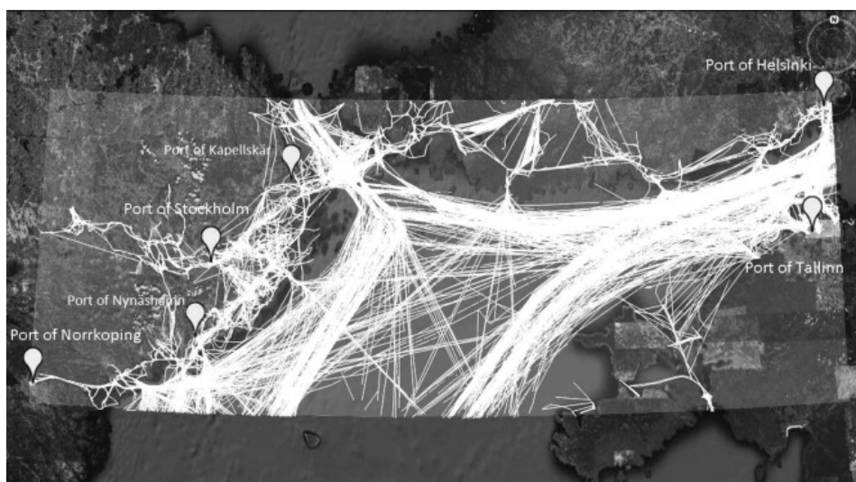
Figure 7.2: The surveillance area and the vessels tracks extracted from AIS data for 6 days. The area is restricted to the north of the Baltic Sea and part of the Gulf of Finland. Ports from left to right are Norrköping, Nynäshamn, Stockholm, Kapellskär, Helsinki and Tallinn (The image is generated by Google Earth).
